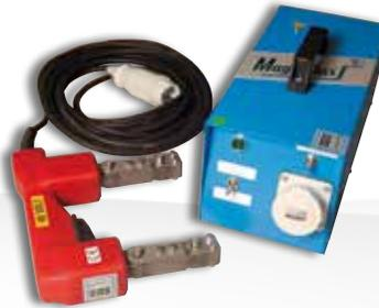
*Electromagnetic Yoke + transformer*
