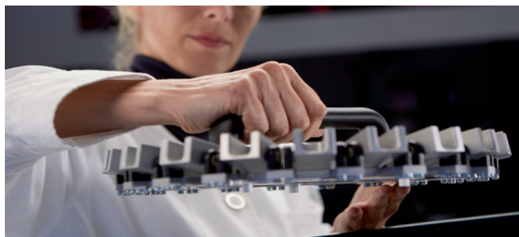
20 position sample tray with failsafe sample chutes
