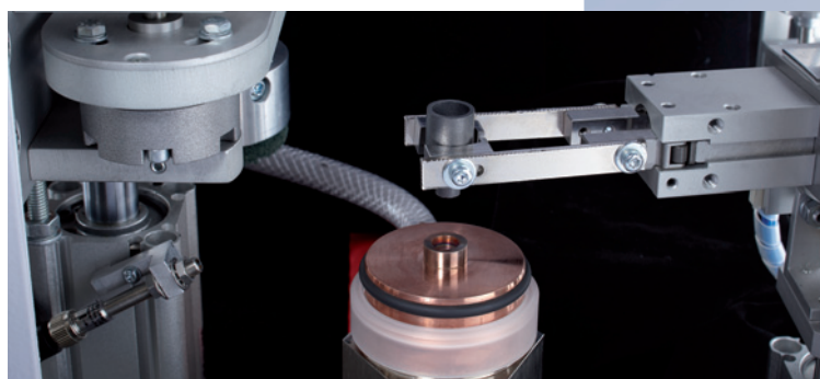
Fully automated crucible handling
