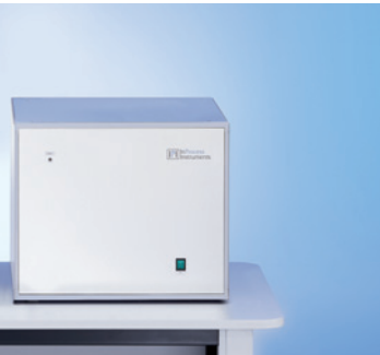
G4 PHOENIX MS with mass spectrometer
