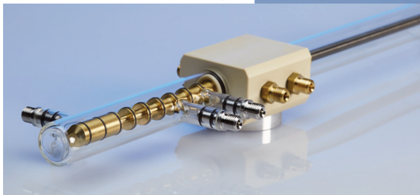
Unique gas calibration unit for standardless hydrogen calibration with 10 independent volumes
