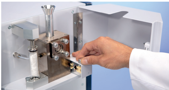
Electrode furnace with SampleCare™ and FusionControl for real-time sample temperature detection, Bruker only.
