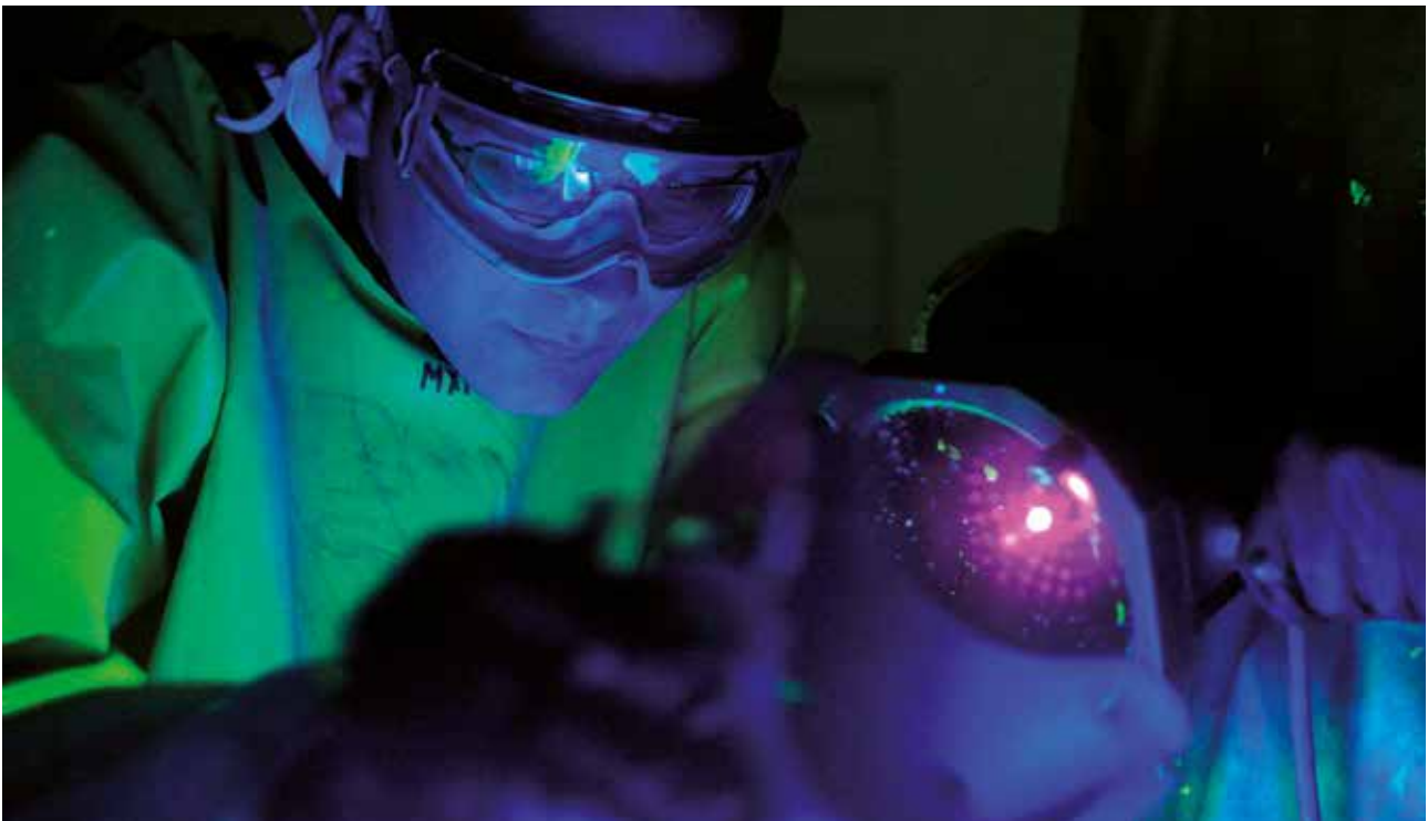
NDI Technician of the 28th Maintenance Squadron inspects a forward support bracket using a Labino 135 Series UV light at the Ellsworth Air Force Base, S.D.
